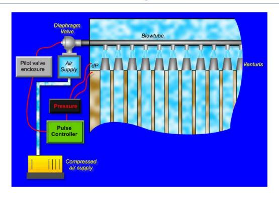
The configuration of the filter cleaning system is crucial to effective filter cleaning and dP control
