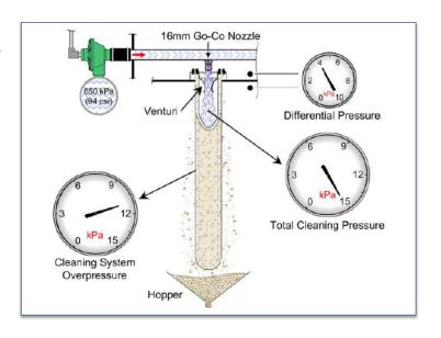
Ample cleaning power, easily adjusted by compressed air pressure level.
