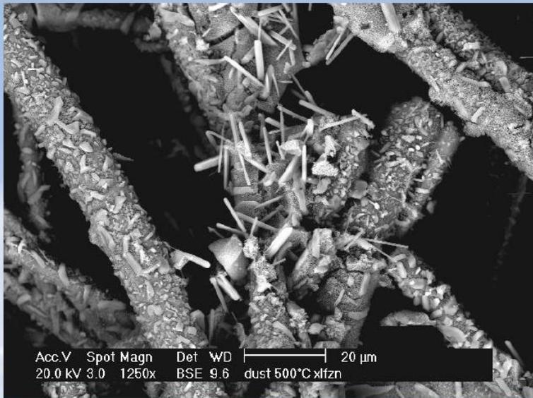
Nano-bits of NO<sub>x</sub>, CO, VOC catalyst are embedded into the walls and adhere to the fibers.
