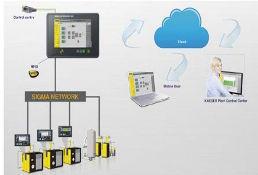
Sigma Air Manager 4.0 is the core of the compressed air station and provides the key technology required to take advantage of future services within the Industry 4.0 operating environment. As the central "brain" of a compressed air system, it assumes control tasks and streams data into the Kaeser Data Center.
