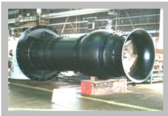
Fixed Vane Circulating Water Pumps
