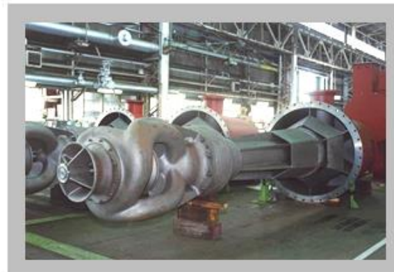
Condensate Extraction Pumps
