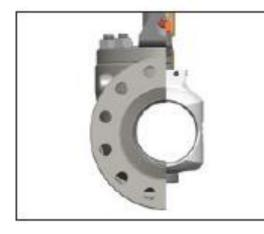
In the fully open position, there is unobstructed flow through the valve.
