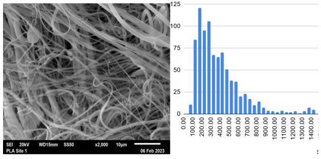
Verdex Technologies has developed and patented a highly scalable and green nanofiber manufacturing process called "melt-film fibrillation" to produce advanced filtration materials. The process can produce materials with fibers as small as 100 nm and submicron pore sizes. The process bears some similarity with meltblown but uses a shearing airflow to produce submicron fibers from a thin film. Unlike electrospinning it is entirely solvent free and produces 3D fibers and a very lofty material.
