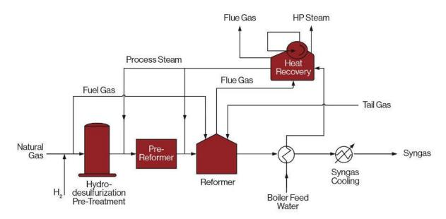
Air Liquide Engineering & Construction provides Steam Methane Reforming (SMR) technology for hydrogen production on both a small and large scale. SMR is a cost-effective and energy efficient way of producing hydrogen. High levels of purity can be reached by employing inhouse Pressure Swing Adsorption purification technology.
