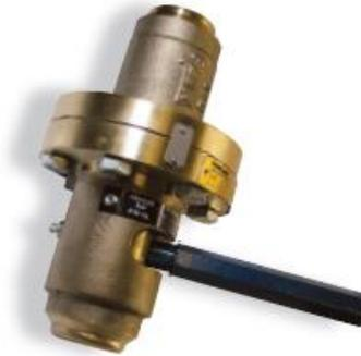
Forum Inline Choke, formerly the Delta Inline Choke, is designed specifically for controlling gas and liquid flowline rates. Water and CO<sub>2</sub> systems are designed to control the rate of fluid injection. The stellite sleeve absorbs the cavitation and pitting action of the fluid as it takes the pressure drop. The sleeve design allows the thickest material around the disc holes and is funnel-shaped to direct the flow back into the center of the piping.
