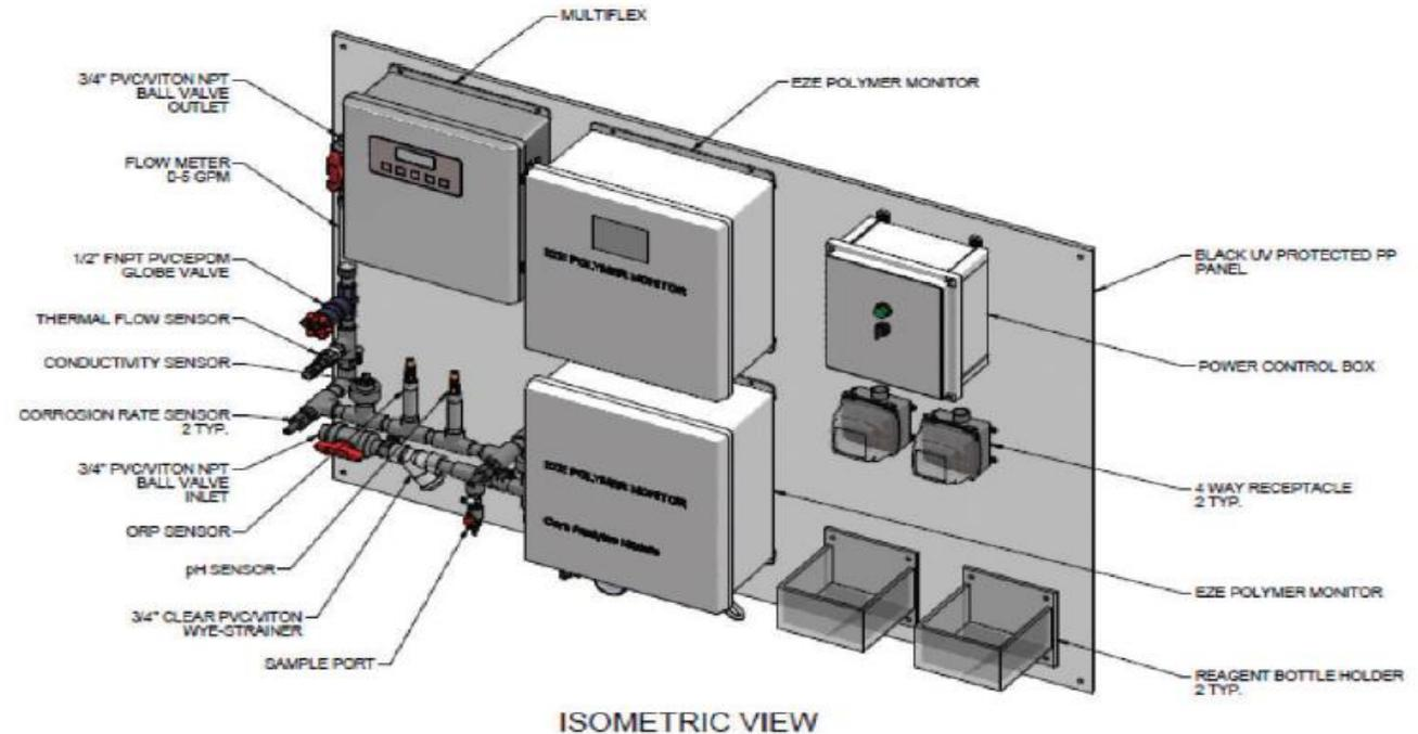
**Figure 1.** Isometric view of EZe Monitor<sup>®</sup> and its components
