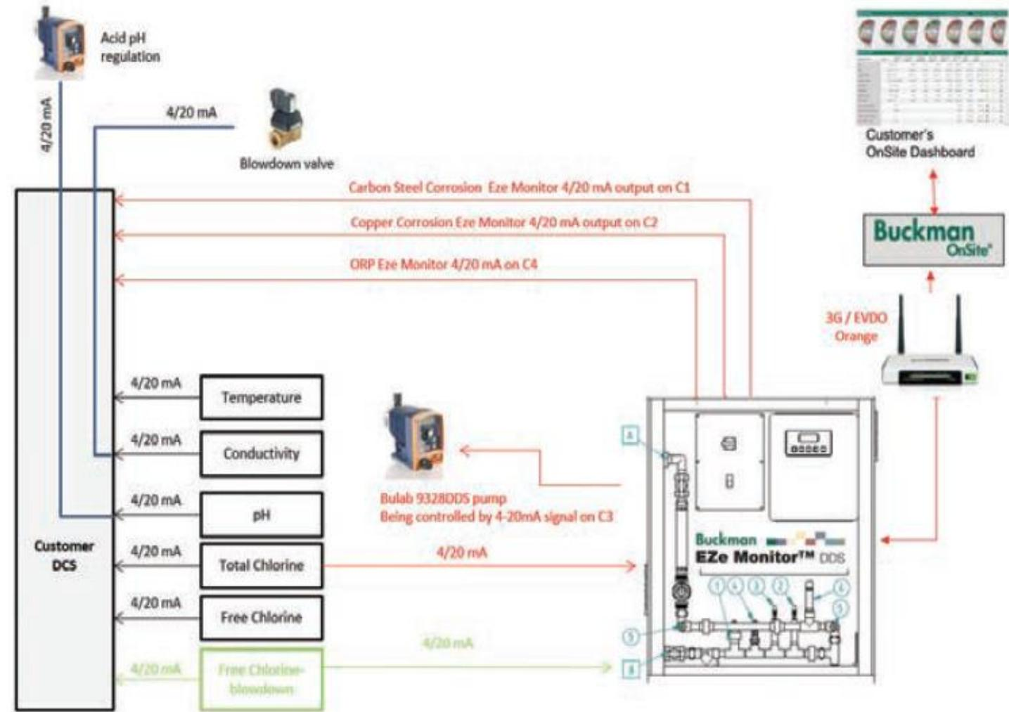
**Figure 4.** A typical system layout diagram of EZe Monitor and OnSite integration
