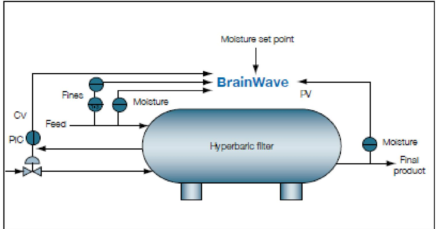
This allows BrainWave to make control corrections as soon as the incoming moisture changes, instead of waiting for the exiting moisture to respond. BrainWave is also able to reduce spikes in air pressure, which cause increased wear and excessive maintenance on equipment. BrainWave accomplishes this by stabilizing the measured moisture content at the filter exit by continuously adjusting air pressure
