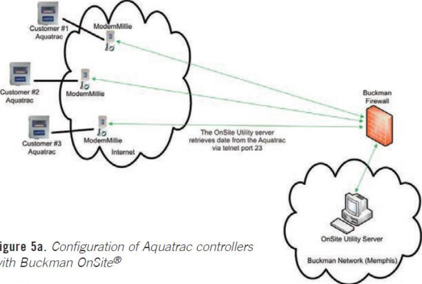
Figure 5a. Configuration of Aquatrac controllers with Buckman OnSite®
